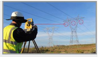
The power of the combined tools allow us to set and measure virtually unlimited spatial points from one location, and also target distances of up to 2000 meters with very high accuracy.
